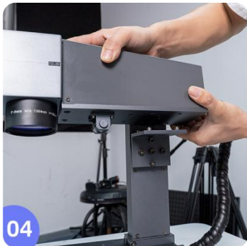
4. Place the lens on the right angle plate of the Y-axis and aim it at the four screw holes in the rear
